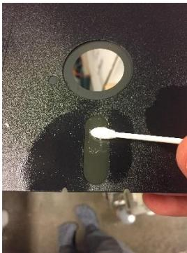
Figure 4: Removing stuck adhesive from media surface with isopropyl alcohol and Q-Tip.
