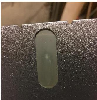
Figure 5: Media damage from removing adhesive
