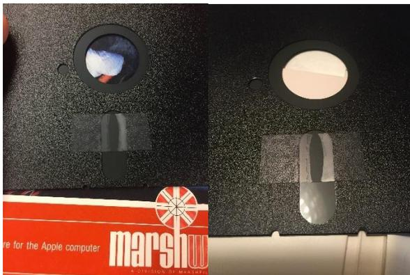
Figure 2: Left: Disk as received with tape on media surface; Right: Closeup of tape on media
